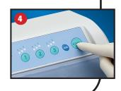
If cleaning a speed increaser or speed reducer, select "EL" Mode for the extra long cleaning cycle. If cleaning a 1:1 attachment, select "L" Mode for the long cleaning cycle. Press the START button and wait until Care3 Plus completes cleaning, lubrication and purging cycle.
