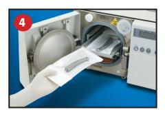
Bag and place motor in the autoclave.
