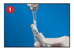
Wash the air motor under warm water and clean softly with a toothbrush.
