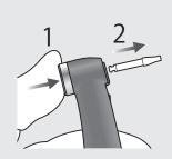
Tighten the screw up securely and then hold down the push button and pull out the guide bur.
