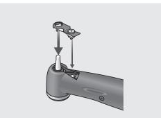
Slide the built-in electrode onto the guide bur and line up the screw holes.
