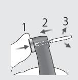
Hold the push button and slide the guide bur straight in as shown in the illustration. Then rotate it left and right.
